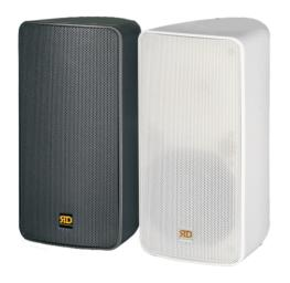
The RD 106T is a highly weather-resistant, single 6" 2-way full range loudspeaker, the body is made of engineering plastic injection molding. fitted with one 6" mid-woofer and one 1" HF driver. The system conforms to IP46 international standard. RD 106T is equipped with multi-tap transformer based on RD 106.
